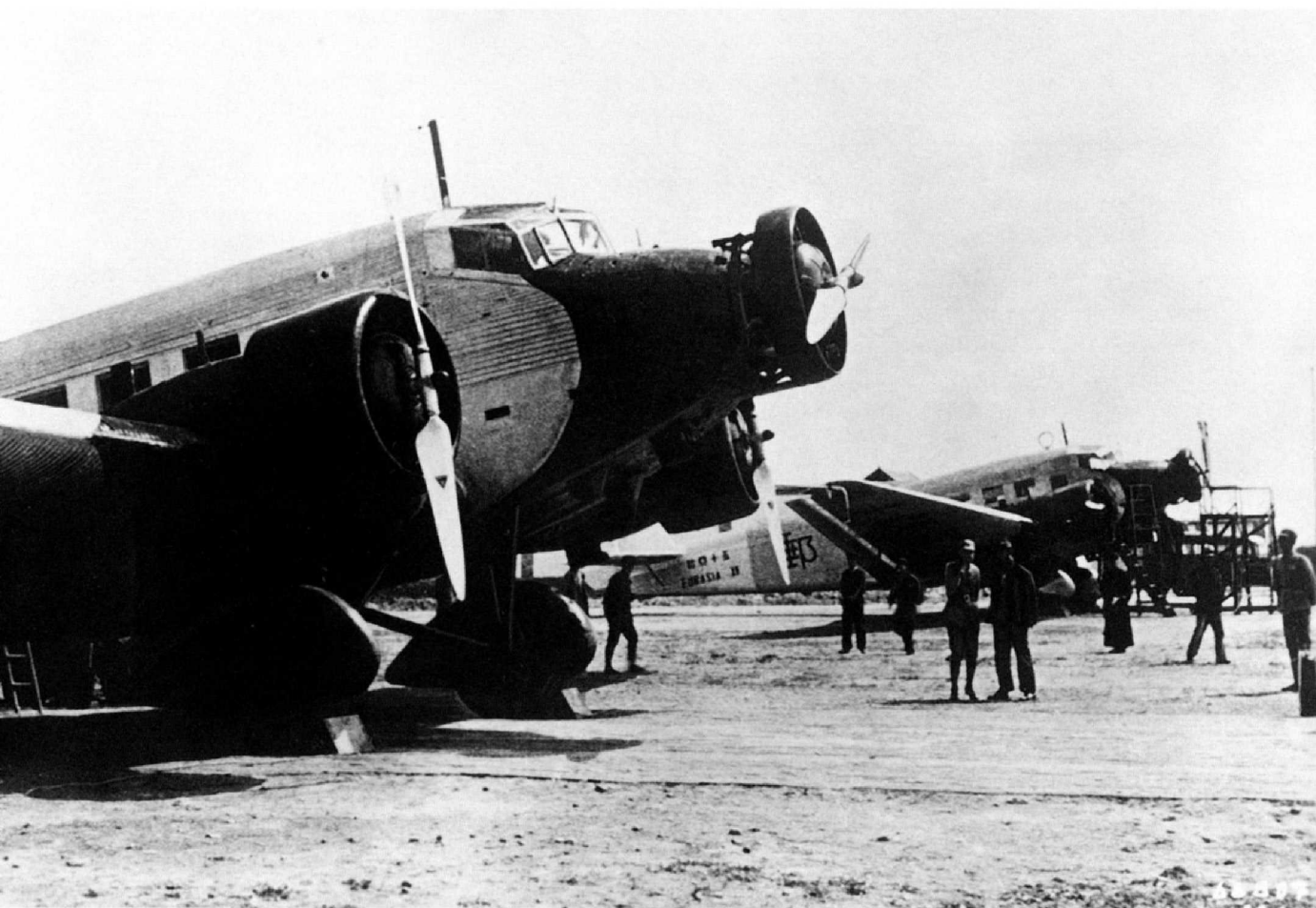
Above: The Junkers Ju 52 was the backbone of the Fallschirmjäger's airlift capacity and is shown here in its civil capacity (where it was a passenger aircraft). Some 4845 of the rugged and reliable "Auntie Jus" or "Iron Annies" were built by Nazi Germany, and they served in a variety of roles: magnetic-mine destroyers, glider tugs, troop transports, freighters and casualty evacuation ambulances. The Ju 52 could carry up to 16 fully equipped paratroopers over a range of 1300km (808 miles) at a speed of 305km/h (190mph).
