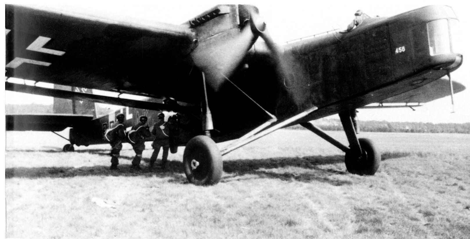
Below: Fallschirmjäger recruits board a Dornier Do 23 bomber for a training jump in the mid-1930s. The Do 23 was one of the first bombers to equip the new Luftwaffe. It was soon discovered that it had many drawbacks, not least being underpowered and beset with handling faults. By 1939 this twin-engined aircraft was obsolete and had been relegated to training duties, such as providing jump platforms for the fledgling airborne arm. Note the external tubular knee pads worn by each jumper. Constructed of leather-covered sponge rubber, they were held in position by a set of two strong elasticated and adjustable straps which crossed behind the knees and clipped onto the button hooks on the opposite side of the pad.
