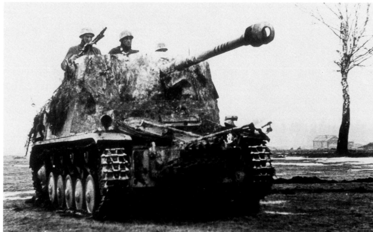
Below: The same vehicle photographed from a different angle. The Marder II was armed with a 75mm Pak 40/2 gun and one MG 34 machine gun. Manned by a crew of three, this particular vehicle has five "kills" to its credit judging by the rings around the barrel of its gun.
